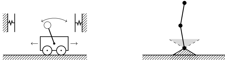
Figure 3: Left: Cartpole with soft walls. Right: Acrobot with soft joint limits.
