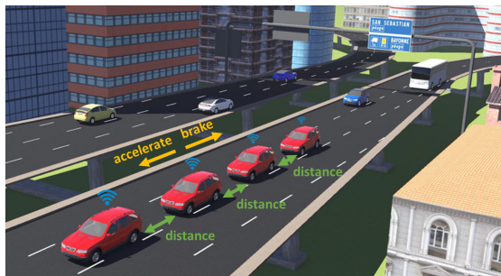
Figure 1: Platoon of self-driving cars (image adapted from Hu et al., 2020).
